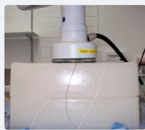
Invasive temperature sensors now can be inserted easily in all desired locations
